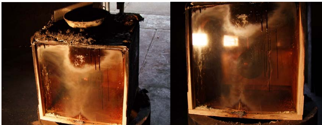
Figure 7 – One Liter Cook Off Test Apparatus after final reaction of IMX-104
