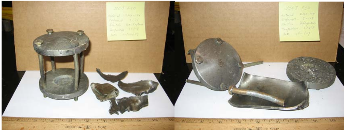
Figure 3: VCCT Fast Cook Off Test Results: 0.075 (pressure rupture) and 0.105 (deflagration)
