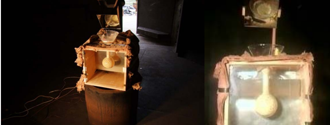
Figure 5 – One Liter Cook-off test setup and appearance of IMX-104 at test start
